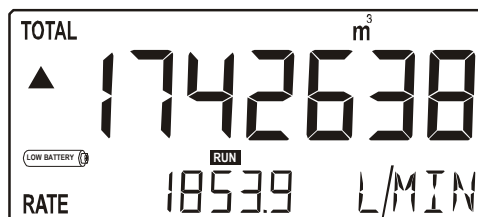
Fig. 4: Example of low-battery alarm.
