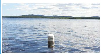
Image: Launched active AB1208 Bath temp buoy
